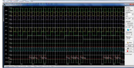
Figure:6 Simulation result of proposed (power consumed=10 \mu w)
