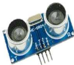
Figure 5: HC-SR04 ULTRASONIC SENSOR
