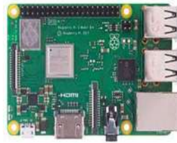
Figure 2: Raspberry Pi 3 Model B+
