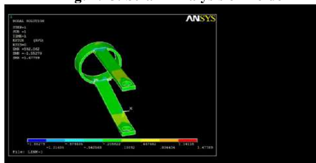
Fig. 7.16: Strain Analysis of Link-1
