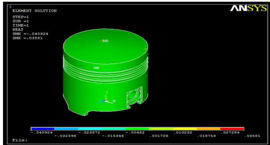
Fig: Heat Flow of Piston – C35 Steel
