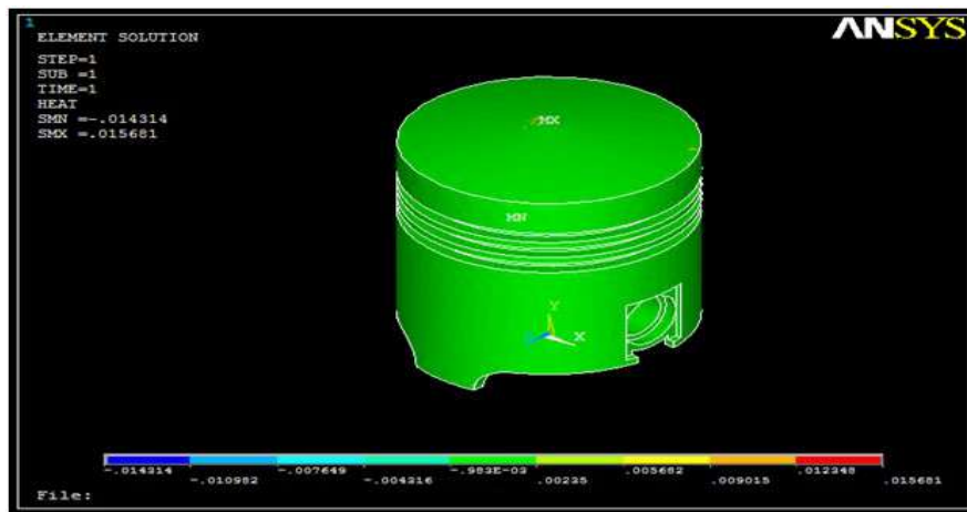
Fig: Heat Flow of Piston – Structural Steel
