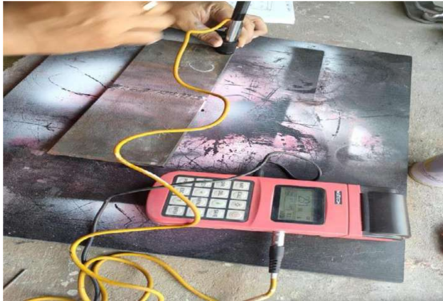
Fig 4.1: Leeb hardness test
