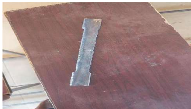
Fig 4.4: Before Testing on UTM
