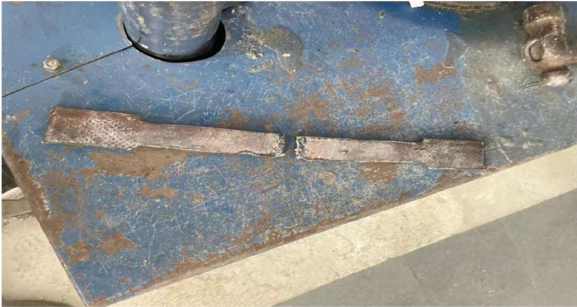
Fig 4.5: After Testing on UTM
