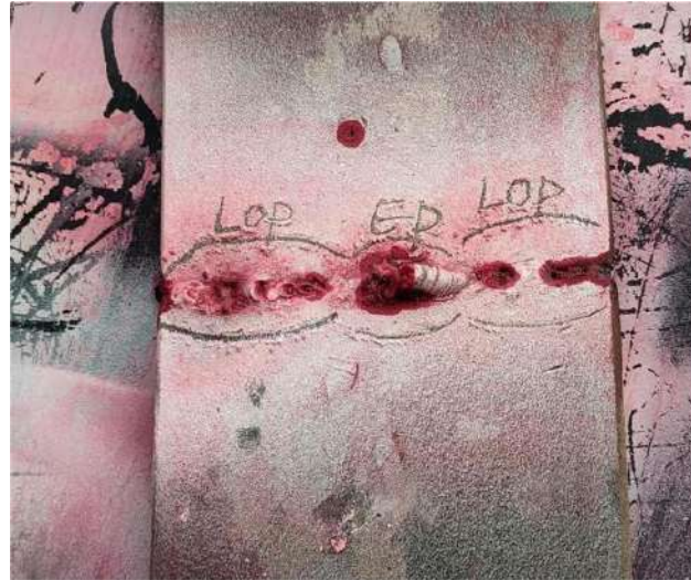
Fig 4.3: Root Side of MS Plate
