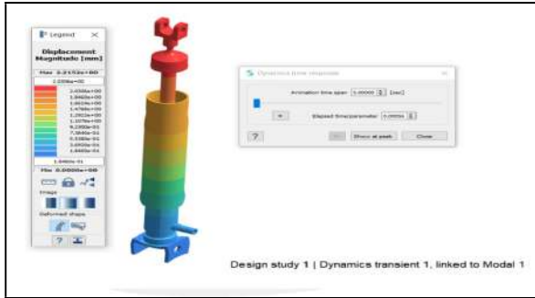
Transient Displacement is 2.215mm
