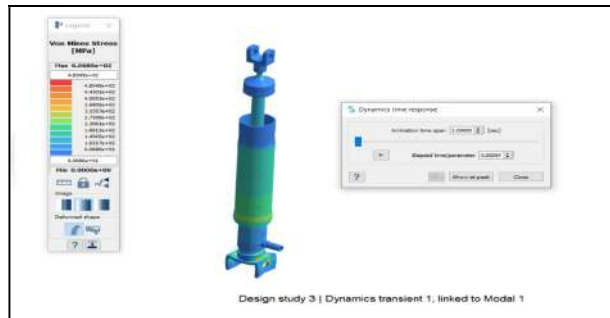
Transient Stress is 485Mpa
