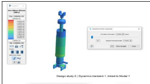
Transient Analysis Stress is 469Mpa
