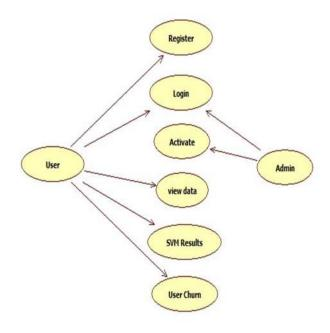
A use case diagram in the Unified Modelling Language (UML) is a type of behavioural diagram defined by and created from a Use-case analysis. Its purpose is to present a graphical overview of the functionality provided by a system in terms of actors, their goals (represented as use cases), and any dependencies between those use cases. The main purpose of a use case diagram is to show what system functions are performed for which actor. Roles of the actors in the system can be depicted.
