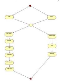
In the Unified Modeling Language, activity diagrams can be used to describe the business and operational step-by-step workflows of components in a system. An activity diagram shows the overall flow of control.
