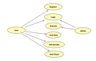
A use case diagram in the Unified Modelling Language (UML) is a type of behavioural diagram defined by and created from a Use-case analysis. Its purpose is to present a graphical overview of the functionality provided by a system in terms of actors, their goals (represented as use cases), and any dependencies between those use cases. The main purpose of a use case diagram is to show what system functions are performed for which actor. Roles of the actors in the system can be depicted.
