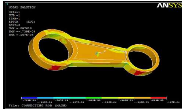
Fig. 7.8: Strain Analysis of Connecting Rod (Magnesium Alloy)
