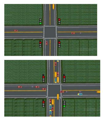
In above screen you can see PYGAME simulation output and at each lane traffic density is calculated and then adjust green and red line. This simulation run in INFINITE loop so you press 'windows' key from keyboard and then close application and then restart and run second YOLO module
