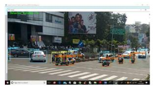
In above screen detecting traffic and then estimating its count and based on that traffic time will be adjusted. YOLO runs very slowly in normal laptop so let it finish all frame processing then u will get output.mp4 file which you can play as normal video with traffic density.
