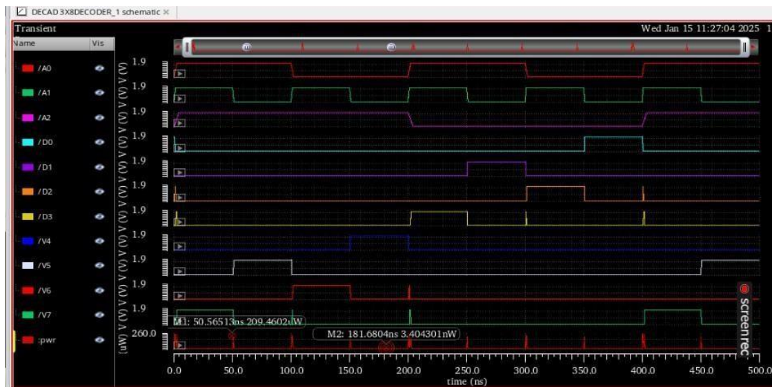
Fig.5: Power analysis of 3x8 decoder with enable pin
