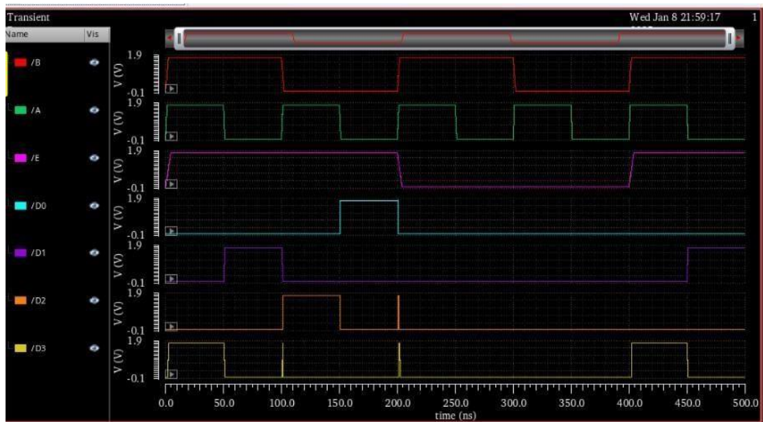
Fig.1: Simulation of 2x4 decoder with enable pin
