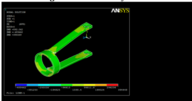
Fig. 7.10: Stress Analysis of Link-1
