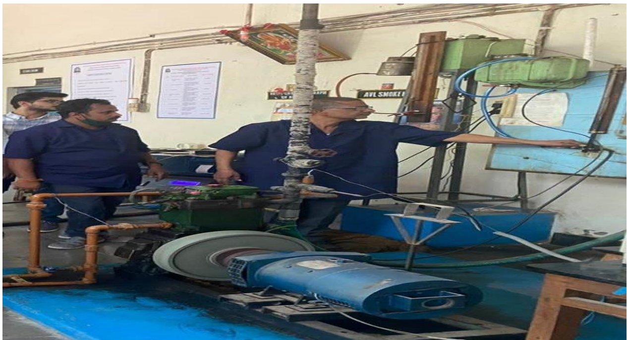
Figure 3. 14 : AVL 437 Smoke Meter (Source : CBIT )
