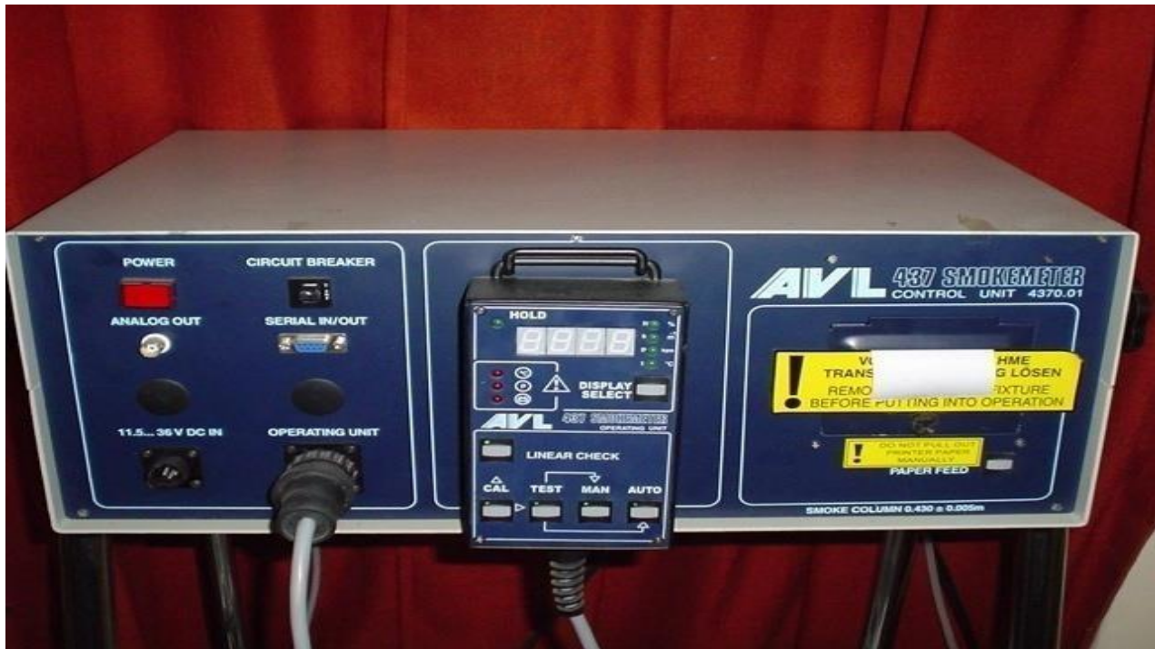
Figure 3. 14 : AVL 437 Smoke Meter (Source : CBIT )
